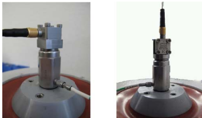
Figure 4 – Mounting a Kistler 8793A500 triaxial accelerometer in z-axis (4a. left) and x-axis (4b. right) to the reference side of a back-to-back reference sensor Kistler 8076K.
